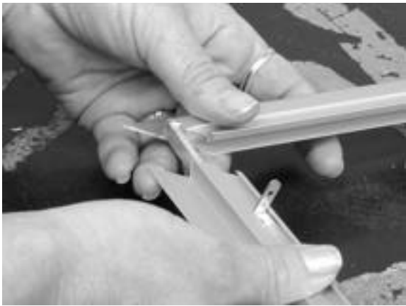
3. The small side of the frame is assembled with the long sides. The hooks are not pressed yet
