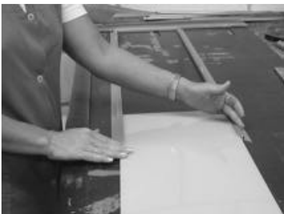
5. The diffuser is glided into the frame.
