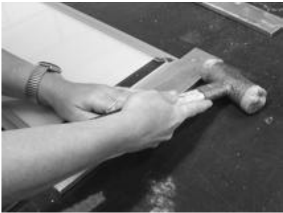
8. The frame is pressed together with a hammer and the use of a protection metal part
